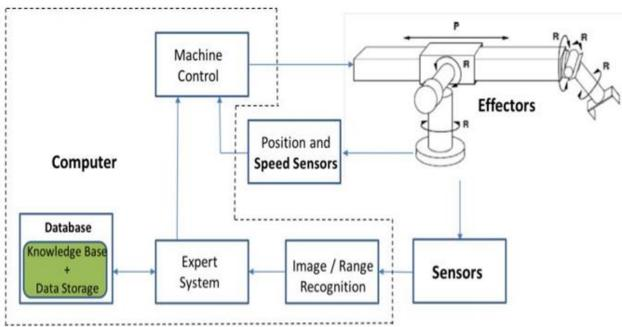
Figure 1. Components of an intelligent robot
